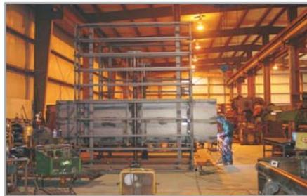
Double Frame Vertical Reciprocating Conveyors are specifically designed for vertical movement of a large, bulky, heavy material from one elevation to another. Requires minimal floor space and easily installed. The model RJS-2 can be surface mounted or placed in a shallow pit. Our RJS-2 model comes with all the same safety features as the RJS model. The RJS-2 has 2 pistons each with dual ANSI chains.
